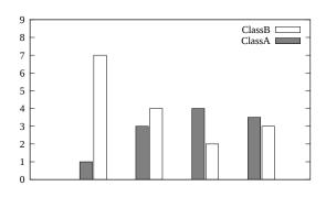
This will produce a plot with clusters of two boxes (vertical bars) centered at each integral value on the x axis. If the first column of the input file contains labels, they may be placed along the x-axis using the variant command
