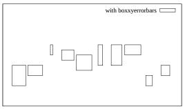
The box width and height are determined from the x and y errors in the same way as they are for the **xyerrorbars** style — either from xlow to xhigh and from ylow to yhigh, or from x-xdelta to x+xdelta and from y-ydelta to y+ydelta, depending on how many data columns are provided.
