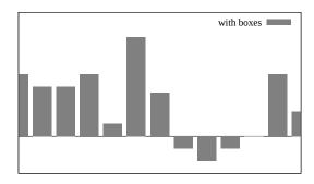
The width of the box is obtained in one of three ways. If the input data has a third column, this will be used to set the width of the box. If not, if a width has been set using the **set boxwidth** command, this will be used. If neither of these is available, the width of each box will be calculated automatically so that it touches the adjacent boxes.
